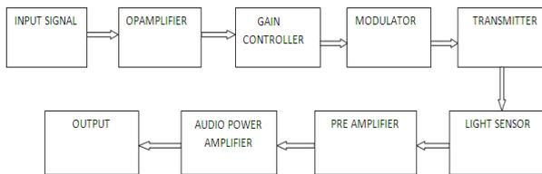
Figure 1: Block diagram of total working order of the system
