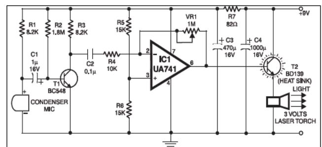
Figure 2: Laser based Voice Transmitter Circuit
