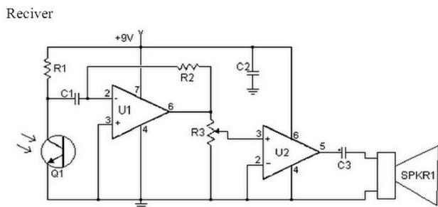
**Figure3: Laser based Voice Receiver Circuit**
